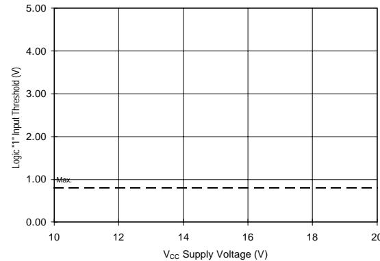
Figure 22B. Logic "1" Input Threshold vs. Voltage
