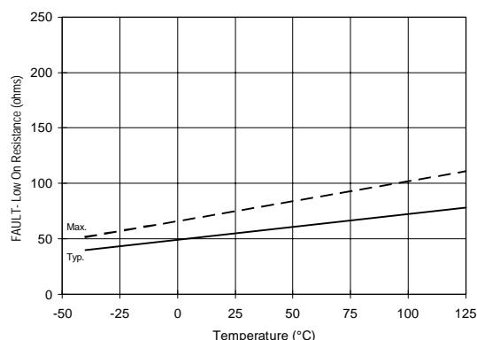
Figure 37A. FAULT Low On Resistance vs. Temperature
