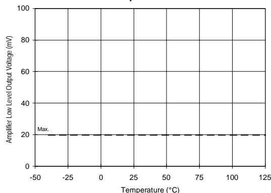
Figure 45A. Amplifier Low Level Output vs. Temperature
