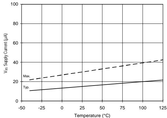
Figure 27A. V<sub>BS</sub> Supply Current vs. Temperature
