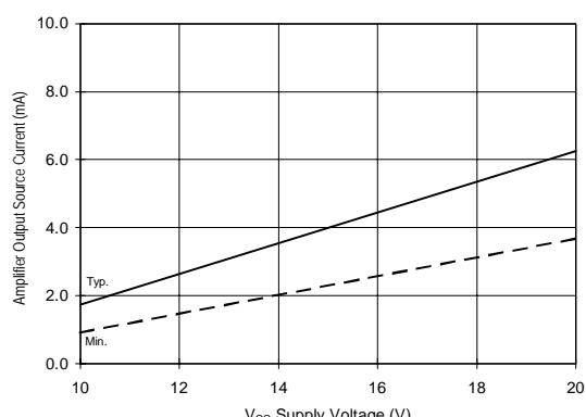
Figure 46B. Amplifier Output Source Current vs. Voltage
