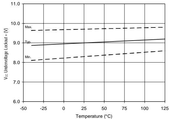
Figure 35. V<sub>CC</sub> Undervoltage (+) vs. Temperature
