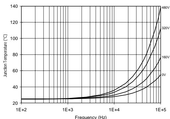
Figure 54. IR2130/IR2132 T<sub>J</sub> vs. Frequency (IRF450)
