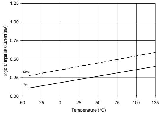
Figure 30A. Logic "0" Input Current vs. Temperature
