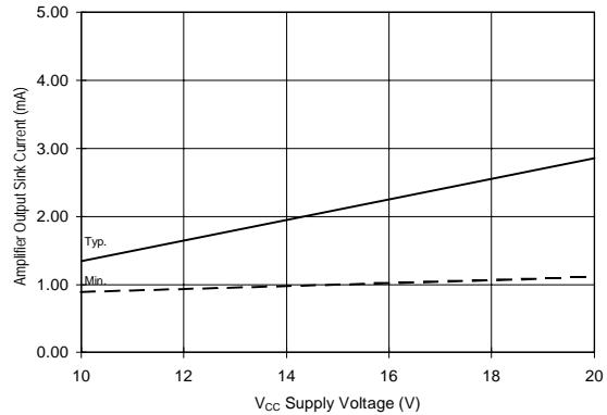
**Figure 47B. Amplifier Output Sink Current vs. Voltage**
