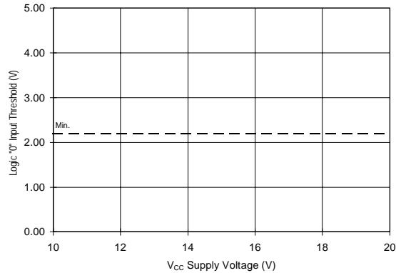
Figure 20B. Logic "0" Input Threshold vs. Voltage
