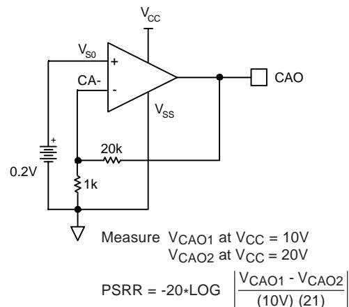
**Figure 10. Operational Amplifier Power Supply Rejection Ratio Measurements**
