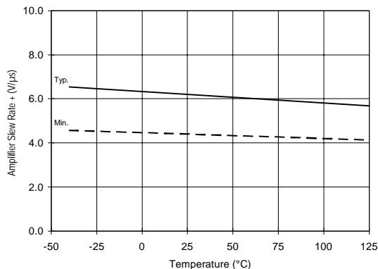
Figure 19A. Amplifier Slew Rate (+) vs. Temperature
