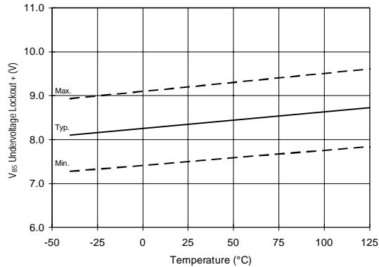
Figure 33. V<sub>BS</sub> Undervoltage (+) vs. Temperature
