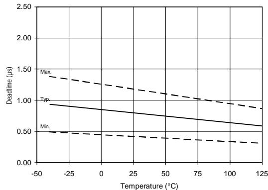
Figure 18C. Deadtime vs. Temperature (IR2132)
