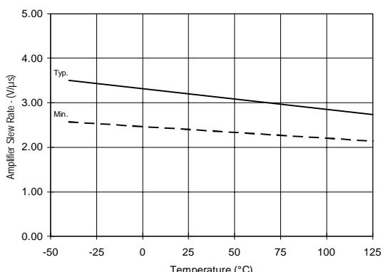
Figure 20A. Amplifier Slew Rate (-) vs. Temperature
