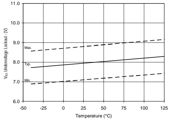
Figure 34. V<sub>BS</sub> Undervoltage (-) vs. Temperature
