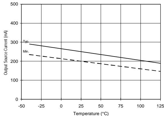
Figure 38A. Output Source Current vs. Temperature
