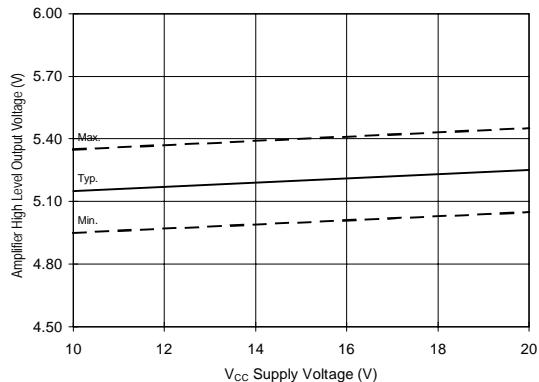
Figure 44B. Amplifier High Level Output vs. Voltage
