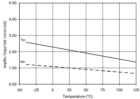
**Figure 47A. Amplifier Output Sink Current vs. Temperature**
