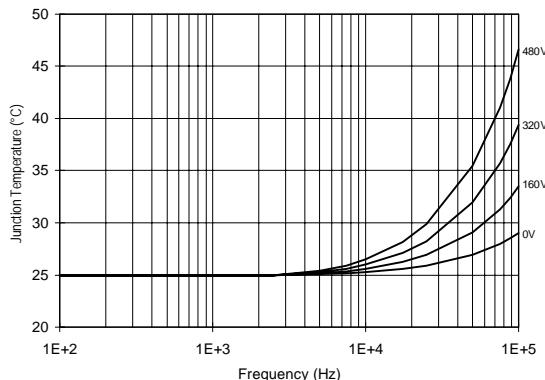
Figure 51. IR2130/IR2132 T<sub>J</sub> vs. Frequency (IRF820)
