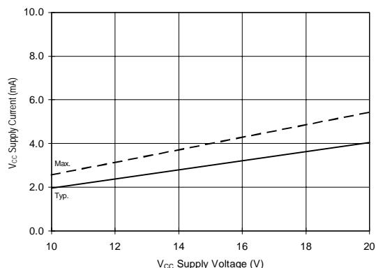
Figure 28B. V<sub>CC</sub> Supply Current vs. Voltage
