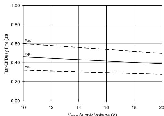
Figure 12B. Turn-Off Time vs. Supply Voltage
