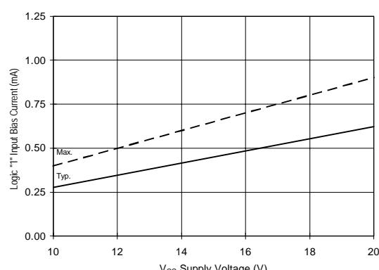
Figure 29A. Logic "1" Input Current vs. Voltage
