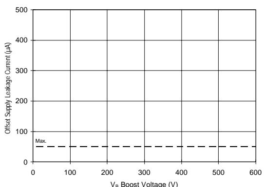
Figure 26B. Offset Supply Leakage Current vs. Voltage
