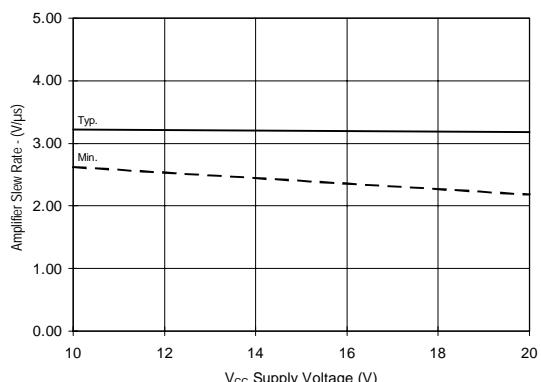
Figure 20B. Amplifier Slew Rate (-) vs. Voltage
