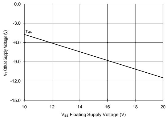
Figure 50. Maximum VS Negative Offset vs. V<sub>BS</sub> Supply Voltage
