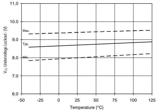
Figure 36. V<sub>CC</sub> Undervoltage (-) vs. Temperature
