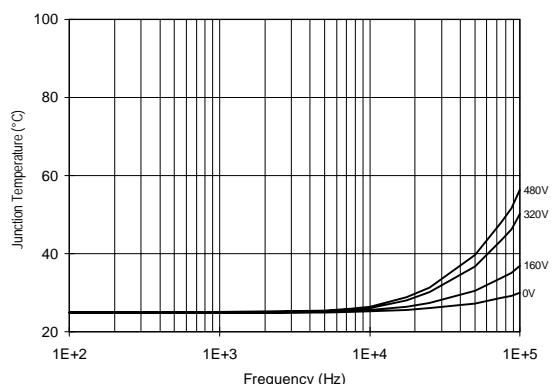
Figure 53. IR2130/IR2132 T<sub>J</sub> vs. Frequency (IRF840)
