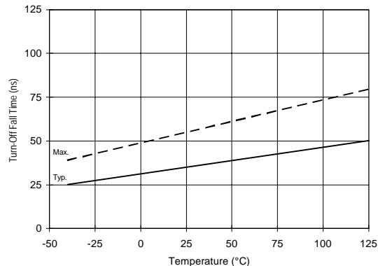
Figure 14A. Turn-Off Fall Time vs. Temperature
