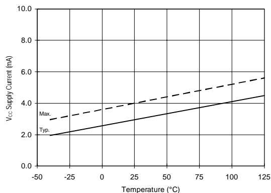
Figure 28A. V<sub>CC</sub> Supply Current vs. Temperature
