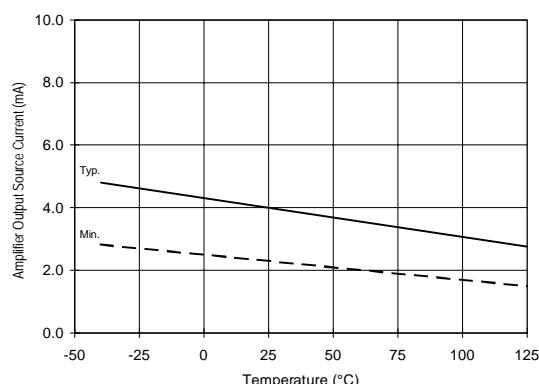
Figure 46A. Amplifier Output Source Current vs. Temperature
