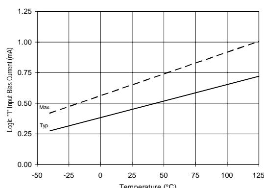
Figure 29A. Logic "1" Input Current vs. Temperature
