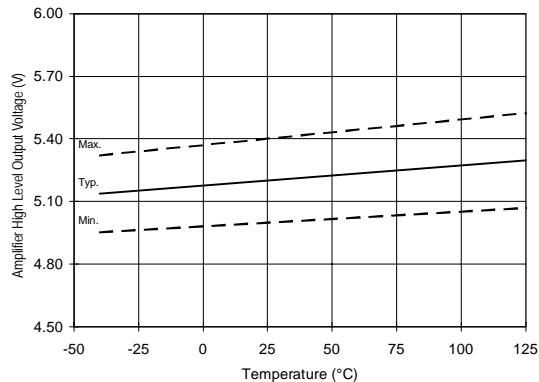
Figure 44A. Amplifier High Level Output vs. Temperature
