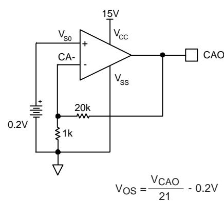
**Figure 8. Operational Amplifier Input Offset Voltage Measurement**
