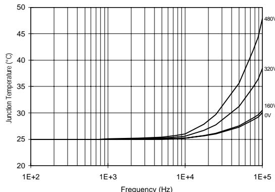
Figure 52. IR2130/IR2132 T<sub>J</sub> vs. Frequency (IRF830)
