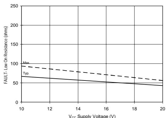
Figure 37B. FAULT Low On Resistance vs. Voltage
