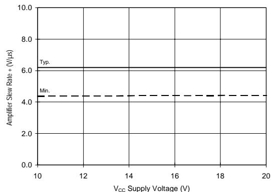
Figure 19B. Amplifier Slew Rate (+) vs. Voltage
