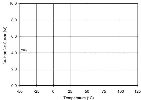
Figure 41A. CA- Input Current vs. Temperature
