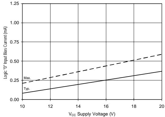
Figure 30B. Logic "0" Input Current vs. Voltage
