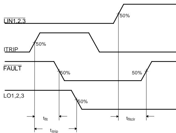
**Figure 5.** Overcurrent Shutdown Switching Time
