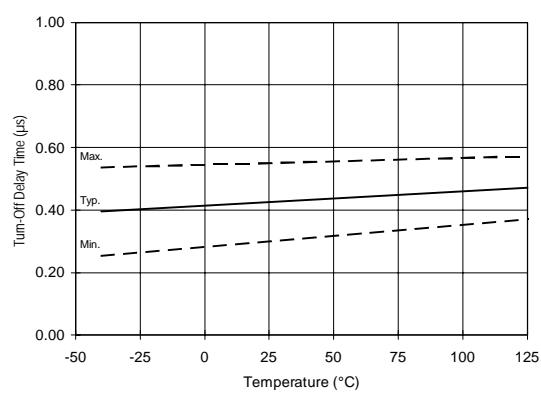
Figure 12A. Turn-Off Time vs. Temperature
