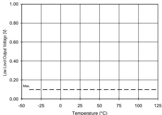
Figure 25A. Low Level Output vs. Temperature
