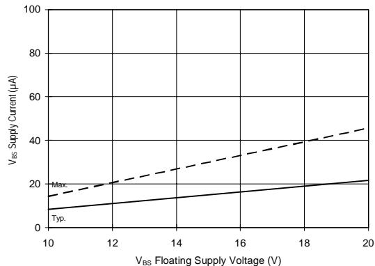
Figure 27B. V<sub>BS</sub> Supply Current vs. Voltage
