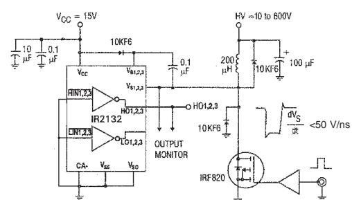
Figure 2. Floating Supply Voltage Transient Test Circuit
