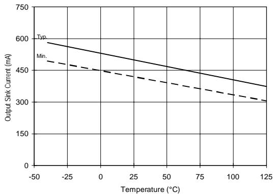
Figure 39A. Output Sink Current vs. Temperature
