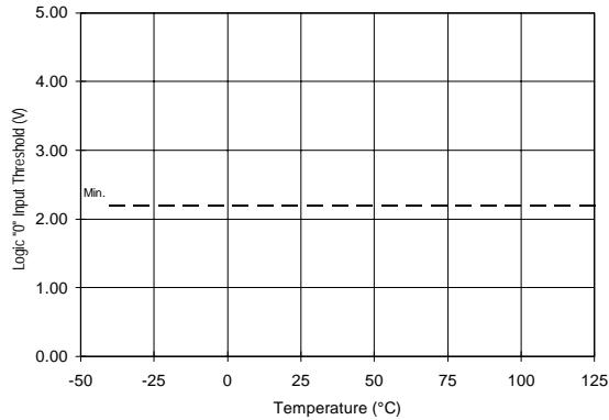
Figure 21A. Logic "0" Input Threshold vs. Temperature
