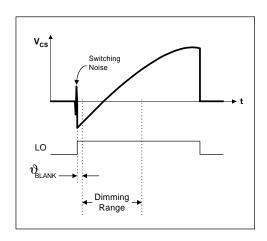
Figure 16, Current sense timing diagram.
