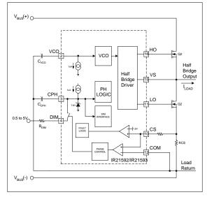
Figure 9, IR21592/IR21593 ignition circuitry.
