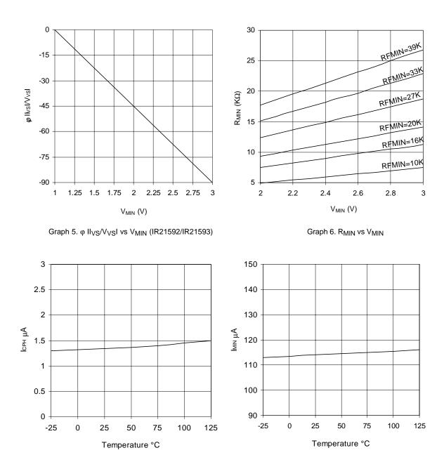
Graph 7. I<sub>CPH</sub> vs Temperature (IR21592/IR21593)
