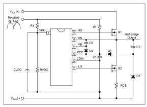
Figure 5, Typical application of start-up circuitry.
