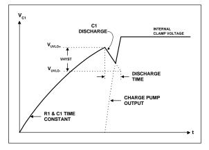
Figure 6, Start-up capacitor (C1) voltage.
