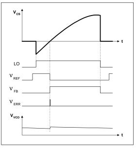
Figure 13, Phase control timing diagram.
