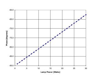
Figure 4, Lamp power vs. phase of output stage.
