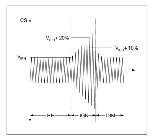
Figure 10, IR21592/IR21593 ignition detection.
