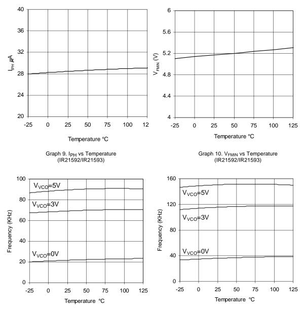
Graph 11. Frequency vs Temperature (IR21592) RFMIN=39K
