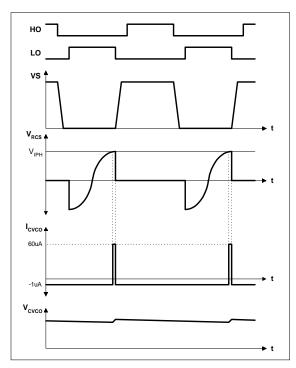
Figure 8, Peak load current regulation timing diagram.
