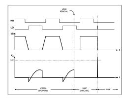
Figure 17, hard-switching with latch off
