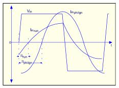
Figure 3, Typical ballast output stage waveforms.
