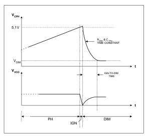
Figure 11, IR21592/IR21593 ignition timing diagram.
