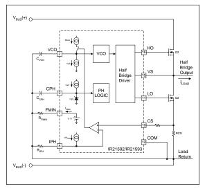
Figure 7, IR21592/IR21593 preheat circuitry.
