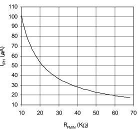
Graph 4. I<sub>IPH</sub> vs R<sub>FMIN</sub> (IR21592/IR21593)
