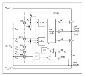
Figure 12, IR21592/IR21593 dimming circuitry.
