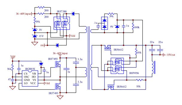
Figure 4 - IR2085S DC Bus converter reference design.
