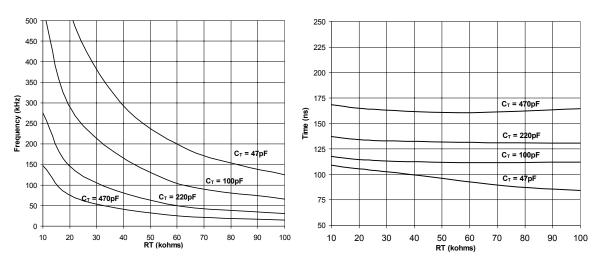
Fig. 1 Typical Output Frequency (-25°C to 125°C)
