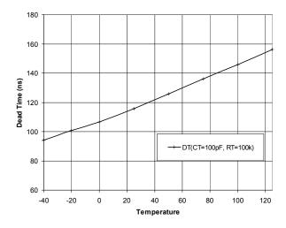
Fig. 3 Typical Dead Time vs Temperature
