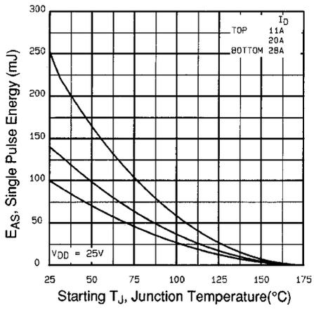
**Fig 13c.** Maximum Avalanche Energy Vs. Drain Current
