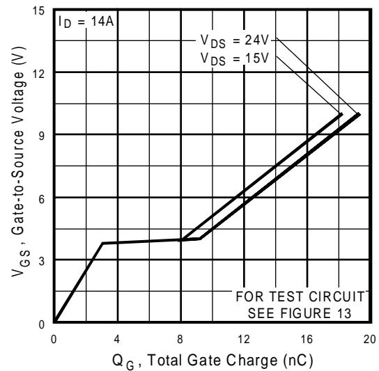
**Fig 6.** Typical Gate Charge Vs.
