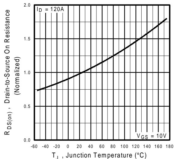
**Fig 4.** Normalized On-Resistance
