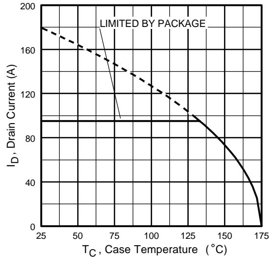
**Fig 9.** Maximum Drain Current Vs.
