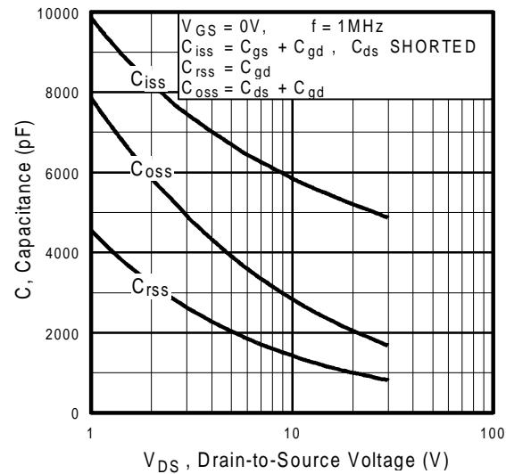
**Fig 5.** Typical Capacitance Vs.
