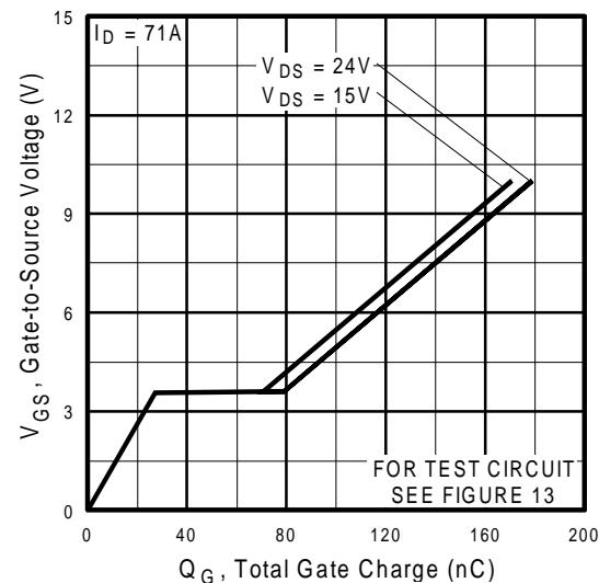
**Fig 6.** Typical Gate Charge Vs.
