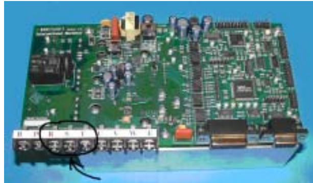
Figure 3. Power Terminal Block, J1
