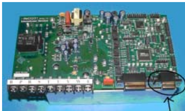
Figure 6. RS232 Connector, J6
