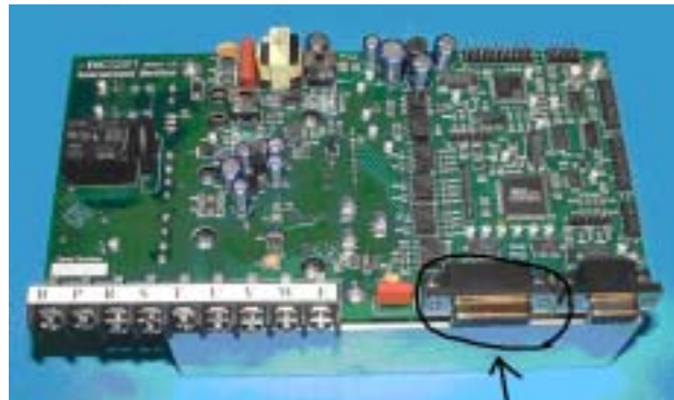
Figure 5. Encoder Connector, J2
