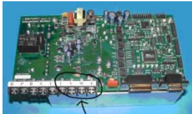
Figure 4. Motor Wiring Connection
