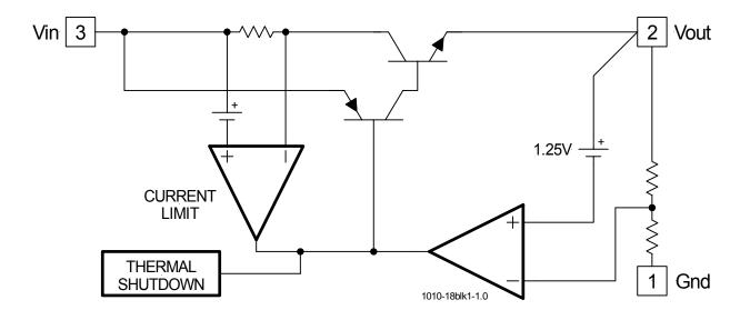
Figure 2 - Simplified block diagram of the IRU1010-18.
