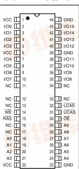
42 GND VCC [ 1/00 41 1/015 1/01 40 1/014 1/02 39 1/013 1/03 38 1/012 vcc [ 37 **GND** I/O4 [ 36 □ I/O11 1/05 35 1/06 34 1 1/09 1/07 33 1/08 10 NC [ 11 32 NC 31 LCAS NC [ 12 30 UCAS WE [ 13 RAS [ 29 OE 14 NC [ 15 28 🛮 A9 NC [ 16 27 🛮 A8 A0 [ 17 26 A7 A1 [ 25 🛮 A6 18 24 🛮 A5 A2 [ 19 АЗ П 20 23 🛮 A4 vcc П 22 GND
