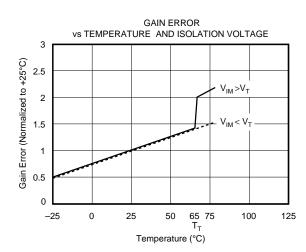
$\label{eq:NOTES: V_T and T_T approximate the threshold} for the indicated gain shift. This is caused by the properties of the optical cavity.$
