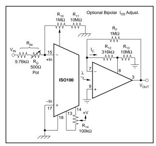
FIGURE 7. Adjusting the Bipolar Errors.
