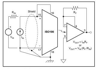
FIGURE 9. Bipolar Noninverting.
