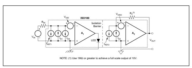
FIGURE 2. Circuit Model for DC Errors in the ISO100.
