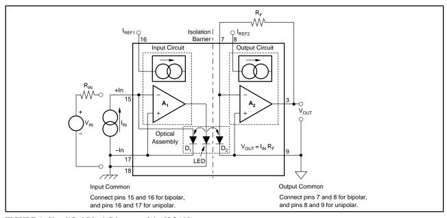
FIGURE 1. Simplified Block Diagram of the ISO100.
