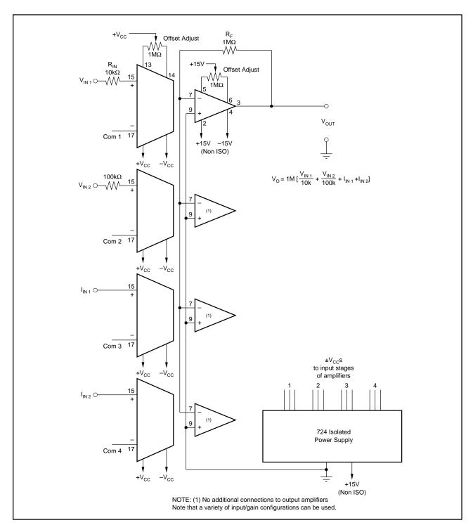
FIGURE 17. Four-Port Isolated Summing Amplifier (Unipolar).
