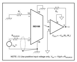
FIGURE 10. Unipolar Inverting.
