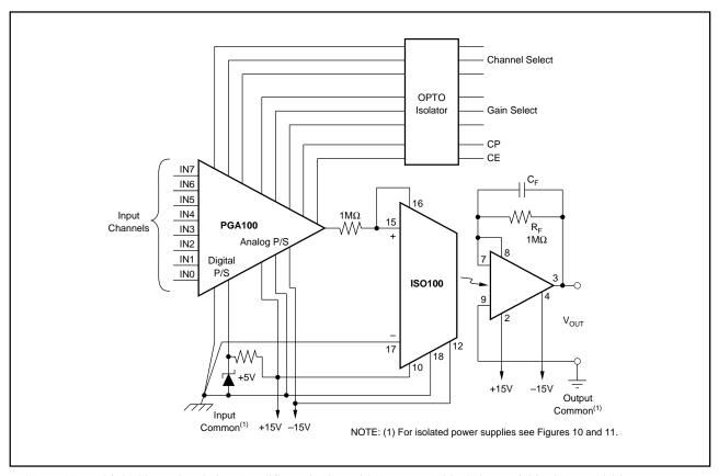
FIGURE 18. Multiple Channel Isolation Amplifier (Bipolar) with Programmable Gain (useful in data acquisition systems).
