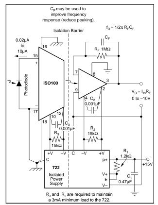
FIGURE 12. Two-Port Isolation Photodiode Amplifier Unipolar.
