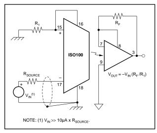
FIGURE 11. Bipolar Inverting.
