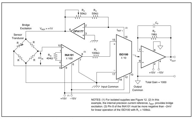
FIGURE 13. Precision Bridge Isolation Amplifier (Unipolar).
