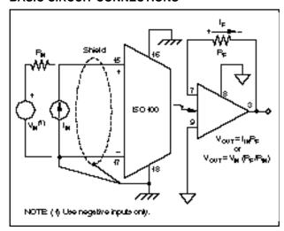
FIGURE 8. Unipolar Noninverting.
