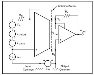
FIGURE 3. High Voltage Error Model.
