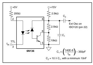
FIGURE 6. Synchronization with Isolated Drive Circuit for Ext Osc Pin.
