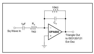
FIGURE 2. Square Wave to Triangle Wave Signal Conditioner for Driving ISO120/121 Ext Osc Pin.
