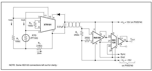
FIGURE 11. Isolated 4-20mA Instrument Loop. (RTD shown).
