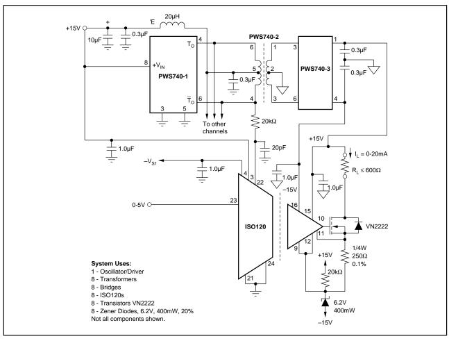
FIGURE 7. Eight-channel Isolated 0-20mA Loop Driver.
