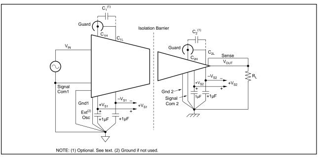
FIGURE 3. Power and Signal Connections.
