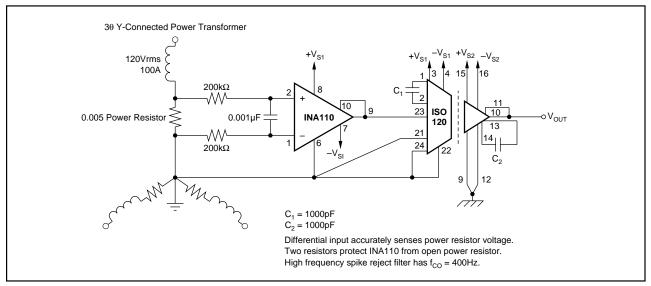
FIGURE 8. Isolated Powerline Monitor.
