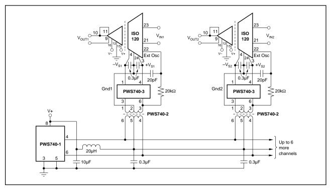
FIGURE 12. Synchronized-Multichannel Isolation System.
