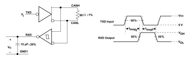
Figure 9. t<sub>LOOP</sub> Test Circuit and Voltage Waveforms
