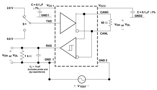
Figure 13. Common-Mode Transient Immunity Test Circuit
