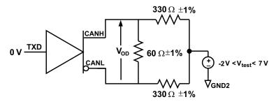
Figure 3. Driver V<sub>OD</sub> with Common-mode Loading Test Circuit
