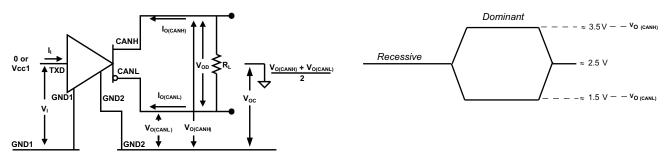
Figure 1. Driver Voltage, Current and Test Definitions
