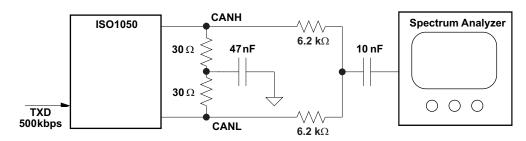
Figure 14. Electromagnetic Emissions Measurement Setup
