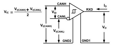
Figure 5. Receiver Voltage and Current Definitions
