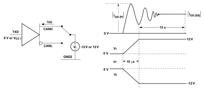
Figure 11. Driver Short-Circuit Current Test Circuit and Waveforms
