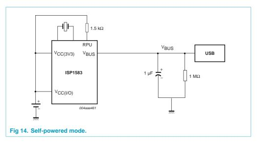
In self-powered mode,  $V_{CC(3V3)}$  and  $V_{CC(I/O)}$  are supplied by the system. Bit SOFTCT in the Mode register must be always logic 1. See Figure 14.
