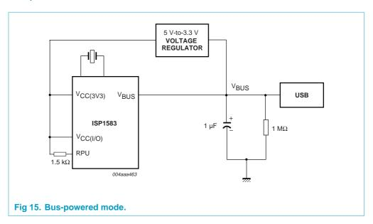
In bus-powered mode (see Figure 15),  $V_{CC(3V3)}$  and  $V_{CC(I/O)}$  are supplied by the output of the 5 V-to-3.3 V voltage regulator. The input to the regulator is from  $V_{BUS}$ . On plugging in of the USB cable, the ISP1583 goes through the power-on reset cycle. In this mode, OTG is disabled.
