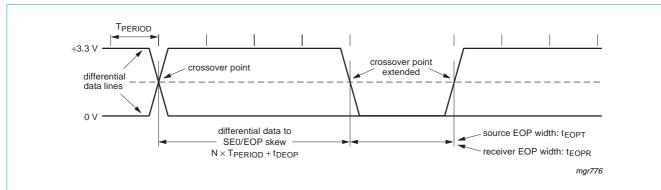
T<sub>PERIOD</sub> is the bit duration corresponding with the USB data rate.
