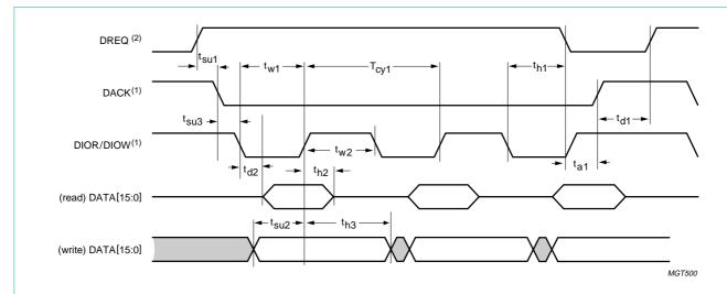
DREQ is continuously asserted until the last transfer is done or the FIFO is full.
