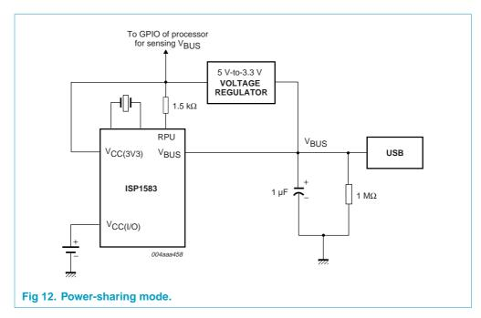
As can be seen in Figure 12, in power-sharing mode,  $V_{CC(3V3)}$  is supplied by the output of the 5 V-to-3.3 V voltage regulator. The input to the regulator is from  $V_{BUS}$ .  $V_{CC(I/O)}$  is supplied through the power source of the system. When the USB cable is plugged in, the ISP1583 goes through the power-on reset cycle. In this mode, OTG is disabled.
