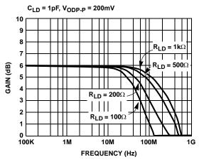
FIGURE 2. SMALL SIGNAL FREQUENCY RESPONSE vs  $R_{\mbox{\scriptsize LD}}$
