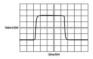
FIGURE 15. SMALL SIGNAL TRANSIENT RESPONSE
