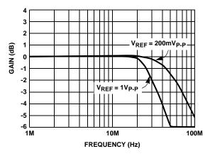
FIGURE 4. FREQUENCY RESPONSE vs V<sub>REF</sub>
