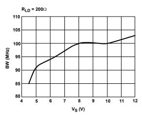
FIGURE 10. BANDWIDTH vs SUPPLY VOLTAGE
