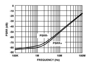
FIGURE 5. POWER SUPPLY REJECTION RATIO vs FREQUENCY
