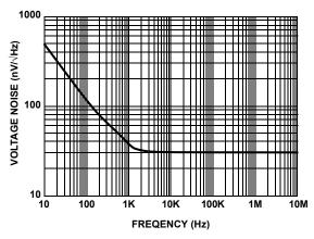
FIGURE 8. INPUT VOLTAGE NOISE vs FREQUENCY
