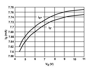
FIGURE 11. SUPPLY CURRENT vs SUPPLY VOLTAGE
