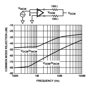
FIGURE 6. COMMON MODE REJECTION vs FREQUENCY
