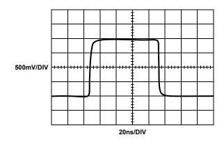
FIGURE 14. LARGE SIGNAL TRANSIENT RESPONSE
