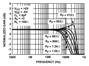
FIGURE 4. FREQUENCY RESPONSE FOR VARIOUS RF
