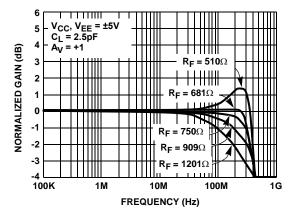
FIGURE 3. FREQUENCY RESPONSE FOR VARIOUS RF
