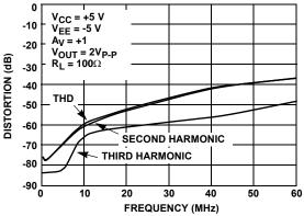
FIGURE 8. DISTORTION vs FREQUENCY (A<sub>V</sub> = +1)
