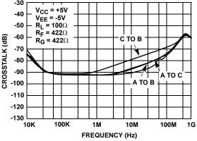
FIGURE 18. CHANNEL CROSSTALK BETWEEN CHANNELS
