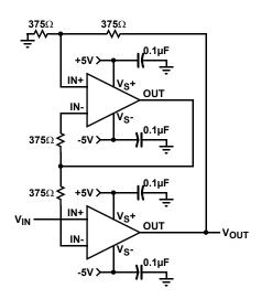
FIGURE 24. FAST-SETTLING PRECISION AMPLIFIER
