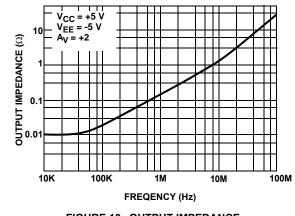
FIGURE 10. OUTPUT IMPEDANCE
