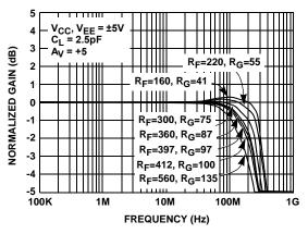
FIGURE 2. FREQUENCY RESPONSE FOR VARIOUS RF
