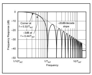
FIGURE 5. Frequency Response of Integrating Converter.
