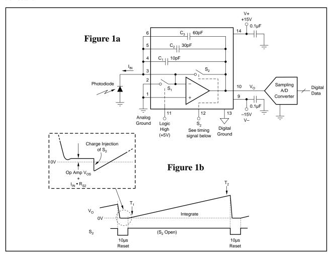
FIGURE 1. Reset-and Integrate Connections and Timing.
