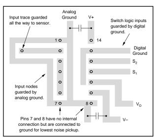
FIGURE 4. Circuit Board Layout Techniques.
