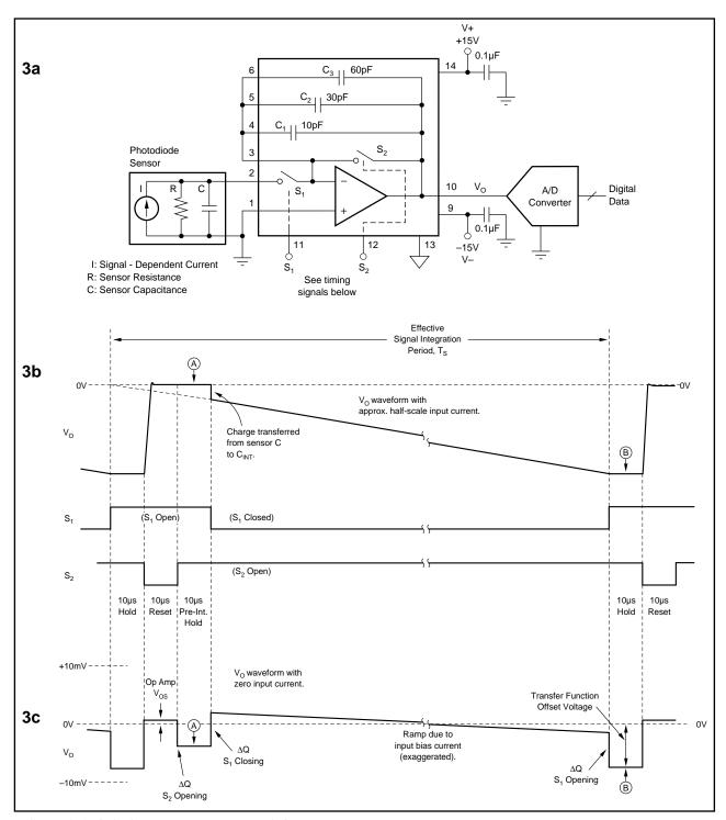
FIGURE 3. Switched-Input Measurement Technique.
