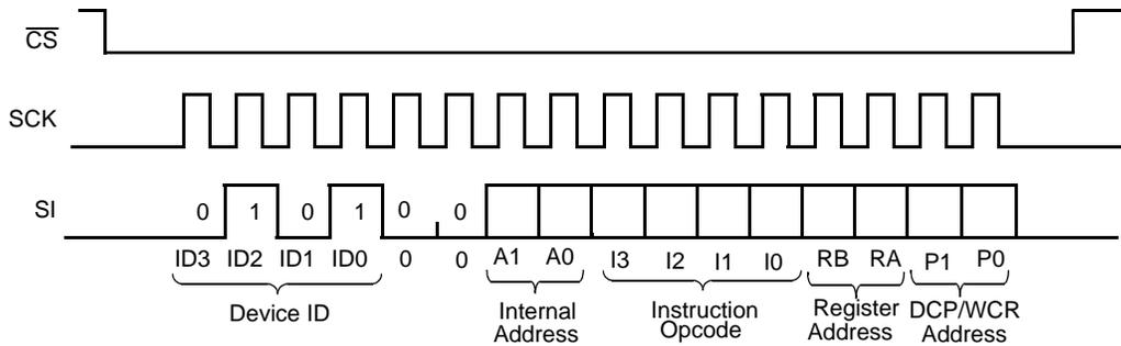
Figure 3. Three-Byte Instruction Sequence SPI Interface; Write Case
