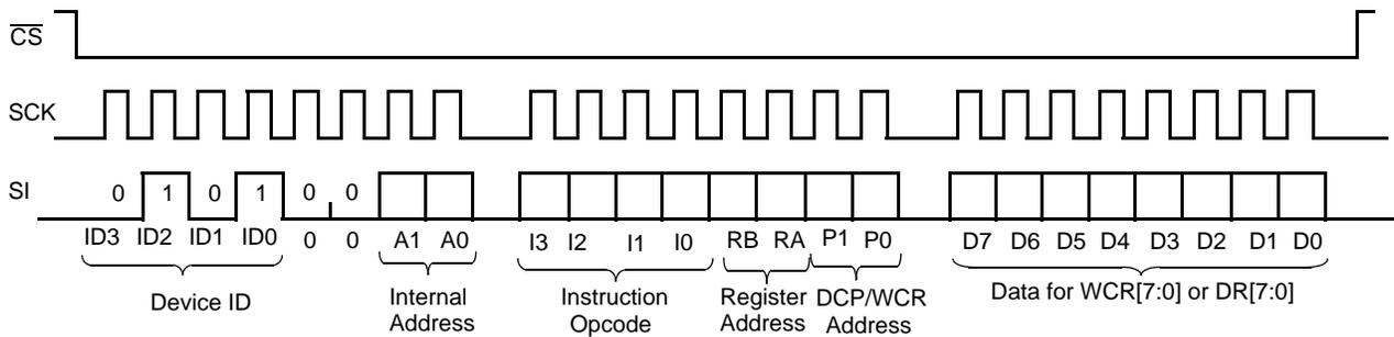
Figure 4. Three-Byte Instruction Sequence SPI Interface, Read Case
