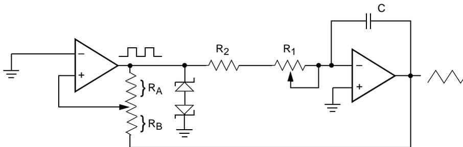
$$\text{frequency} \propto R_1, R_2, C$$
