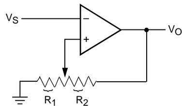
$$V_{UL} = \{R_1/(R_1+R_2)\} V_O(\text{max})$$
