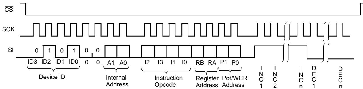
**Figure 7. Increment/Decrement Timing Spec**
