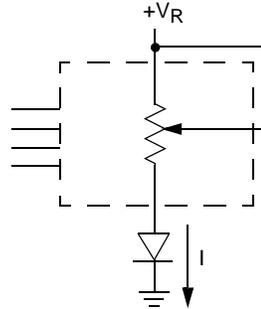
Two terminal Variable Resistor;
