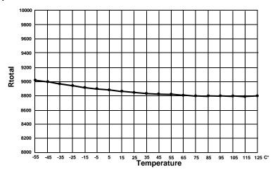
Typical Total Resistance Temperature Coefficient
