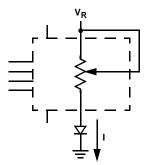
Two terminal variable resistor; variable current
