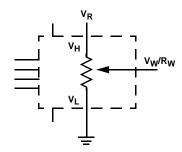
Three terminal potentiometer; variable voltage divider
