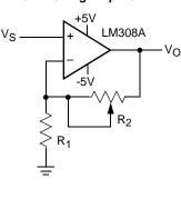
$$V_0 = (1 + R_2/R_1)V_S$$
