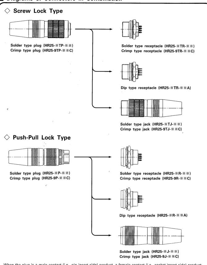
When the plug is a male contact (i.e., pin insert side) product, a female contact (i.e., socket insert side) product should be used for receptacles and jacks. Conversely, when the plug is a female contact (i.e., socket insert side) product, a male contact (i.e., pin insert side) product should be used for receptacles and jacks.
