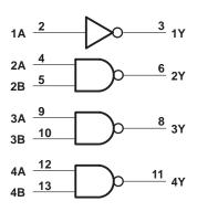
Positive logic  $Y = \overline{A} (\text{driver 1})$   $Y = \overline{AB} \text{ or } \overline{A} + \overline{B} (\text{drivers 2 thru 4})$
