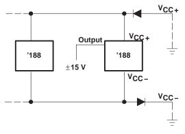
Diodes placed in series with the  $\text{V}_{CC+}$  and  $\text{V}_{CC-}$  leads protect the SN55188/SN75188 in the fault condition in which the device outputs are shorted to  $\pm 15$  V, and the power supplies are at low voltage and provide low-impedance paths to ground.
