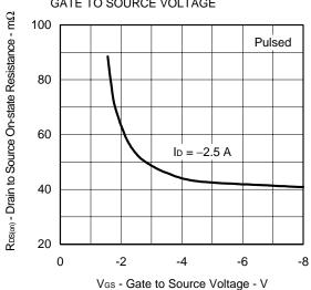
$R_{DS(m)}$  - Drain to Source On-state Resistance -  $m\Omega$
