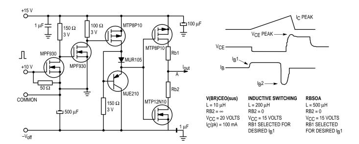
**Table 1. Inductive Load Switching Drive Circuit**
