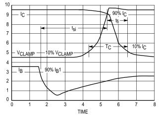
Figure 18. Dynamic Saturation Voltage Measurements
