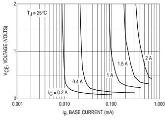
Figure 3. Collector Saturation Region
