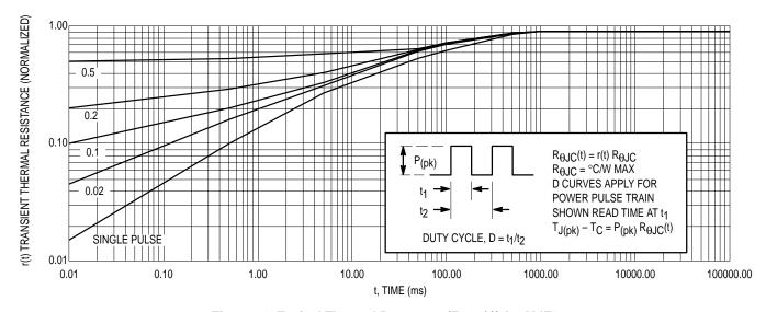
Figure 21. Typical Thermal Response ( $Z_{\theta JC}(t)$ ) for MJF18002
