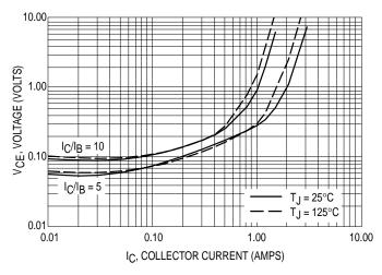
Figure 4. Collector-Emitter Saturation Voltage
