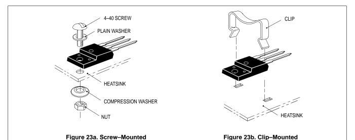
Figure 23. Typical Mounting Techniques for Isolated Package
