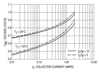
Figure 5. Base-Emitter Saturation Region
