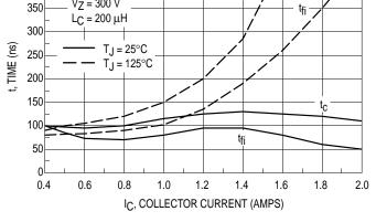
Figure 11. Inductive Switching,  $t_C \& t_{fi}$ ,  $I_C/I_B = 5$
