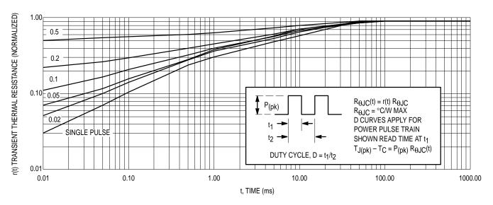
Figure 20. Typical Thermal Response ( $Z_{\theta JC}(t)$ ) for MJE18002
