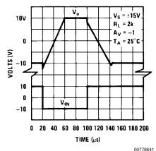
Positive Common-Mode Input Voltage Limit
