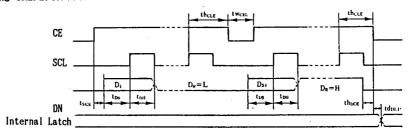
The data is latched at  $D_{\text{\tiny R}}\text{=H}$  and falling edge of the CE signal condition.
