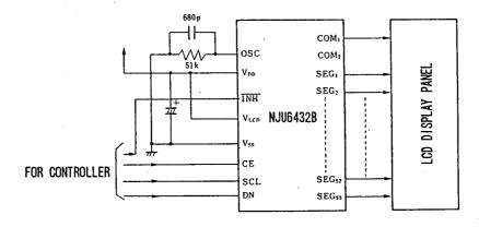
(Note) After rising edge of V<sub>DD</sub> voltage, the display data is not guaranteed and which blinking is meaningless display. Therefore, keep TNH terminal to Low Level by the display data transferred is needed.
