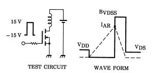
$$\begin{split} R_G &= 25~\Omega \\ V_{DD} &= 90~V,~L = 357~\mu H \end{split}$$
