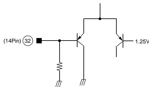
Forward mode:  $V_{FRCTL} \geq 1.8V$
