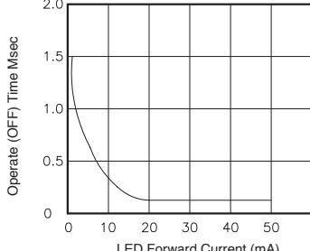
**Fig.11** LED forward current vs. reverse (ON) time
