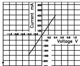
**Fig.9** Off state leakage current
