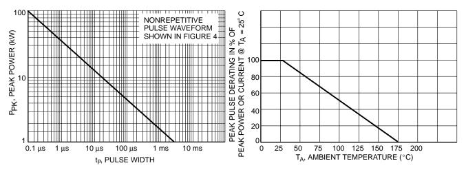
Figure 1. Pulse Rating Curve
