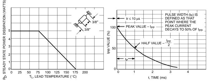
Figure 3. Steady State Power Derating
