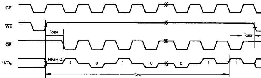
\* During the write cycle, I/O<sub>6</sub> will toggle between "1" and "0".
