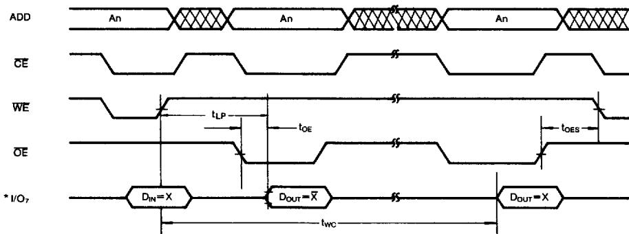
\* During the write cycle, I/O<sub>7</sub> will produce an inverted data of the last I/O<sub>7</sub> data, loaded into the EEPROM
