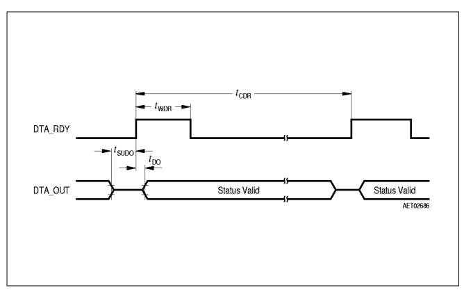
Figure 5 DTA\_RDY Timing Diagram
