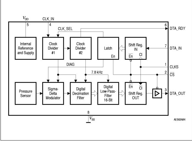
Figure 2 Block Diagram of the KP100
