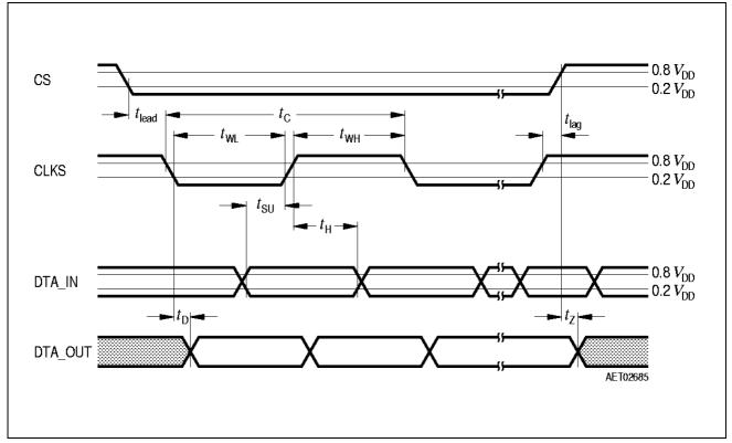
Figure 4 Serial Peripheral Interface: Timing Diagram
