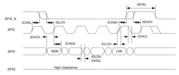
Figure 20. SPI Input Timing
