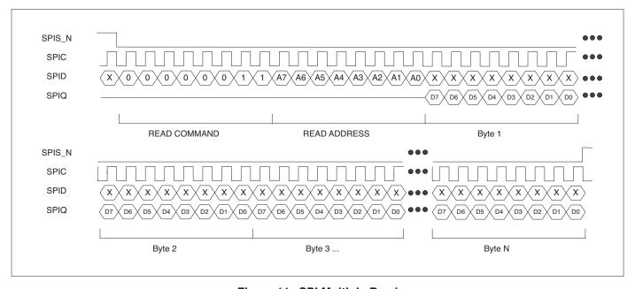
Figure 11. SPI Multiple Read
