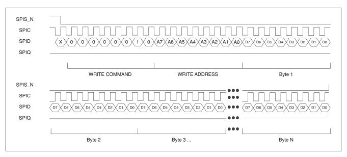
Figure 10. SPI Multiple Write
