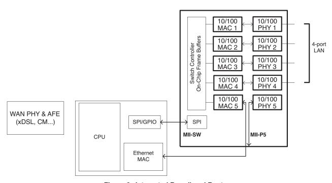
Figure 2. Integrated Broadband Router
