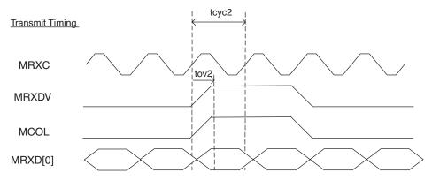
Figure 15. SNI Output Timing
