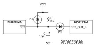
Figure 23. Recommended Reset Circuit.
