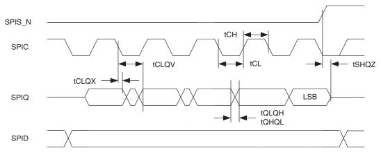
Figure 21. SPI Output Timing
