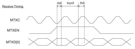
Figure 14. SNI Input Timing
