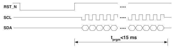
Figure 7. KS8995MA EEPROM Configuration Timing Diagram
