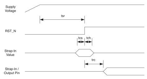
Figure 22. Reset Timing
