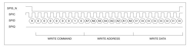
Figure 8. SPI Write Data Cycle
