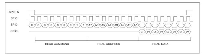
Figure 9. SPI Read Data Cycle
