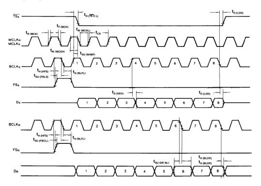
Fig. 2. Short Frame Sync Timing
