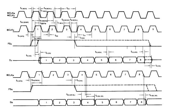
Fig. 3 Long Frame Sync Timing
