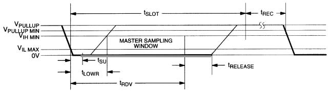
$60 \ \mu s \le t_{SLOT} < 120 \ \mu s$   $1 \ \mu s \le t_{LOWR} < 15 \ \mu s$   $0 \le t_{RELEASE} < 45 \ \mu s$   $1 \ \mu s \le t_{REC} < \infty$   $t_{RDV} = 15 \ \mu s$   $t_{SU} < 1 \ \mu s$
