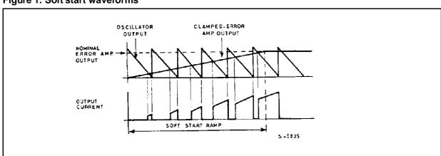
Figure 1. Soft start waveforms
