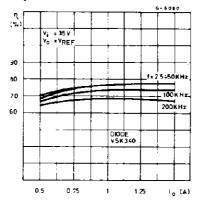
Figure 21. Efficiency vs. output current
