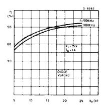
Figure 23. Efficiency vs. output voltage
