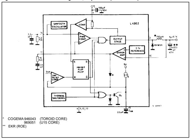
Figure 28. Programmable power supply
