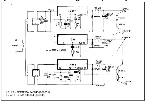
Figure 30. In multiple supplies several L4962s can be synchronized as shown
