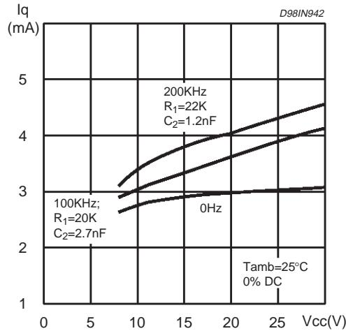
**Figure 5. Stand-by drain current vs. input voltage**
