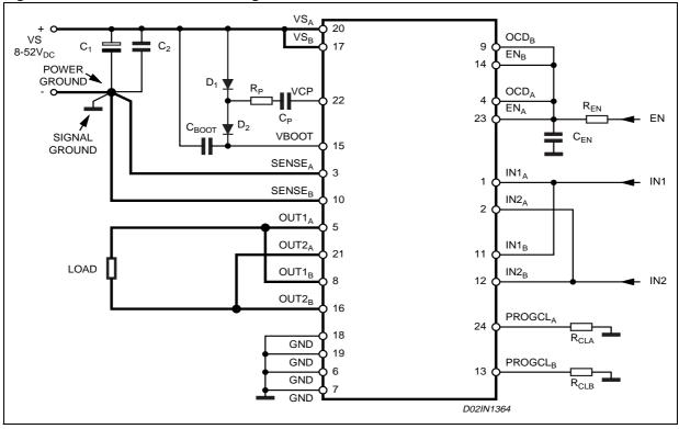
To operate the device in parallel and maintain a lower over current threshold, Half Bridge 1 and the Half Bridge 2 of the Bridge A can be connected in parallel and the same done for the Bridge B as shown in Figure 14. In this configuration, the peak current for each half bridge is still limited by the bond wires for the supply and sense pins so the dissipation in the device will be reduced, but the peak current rating is not increased.
