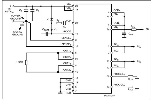
It is also possible to parallel the four Half Bridges to obtain a simple Half Bridge as shown in Fig. 15. In this configuration the, the over current threshold is equal to twice the minimum threshold set by the resistors  $R_{CLA}$  or  $R_{CLB}$  in Figure 15. It is recommended to use  $R_{CLA} = R_{CLB}$ .
