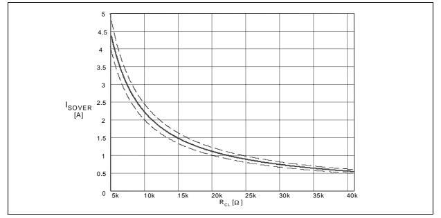
Figure 9. Output Current Protection Threshold versus  $R_{\text{CL}}$  Value
