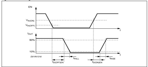
Figure 1. Switching Characteristic Definition
