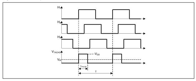
Figure 18. Tachometer Speed Control Loop.
