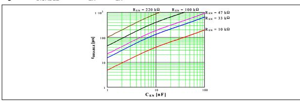
Figure 23.  $t_{DELAY}$  versus  $C_{EN}$ .
