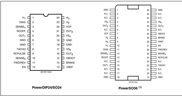
Figure 3. Pin Connections (Top view)
