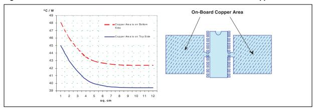
Figure 28. SO24 Junction-Ambient thermal resistance versus on-board copper area.
