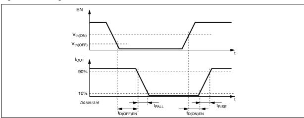
**Figure 5. Overcurrent Detection Timing Definition**
