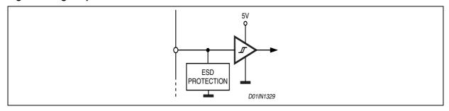
Figure 8. Pin EN Open Collector Driving
