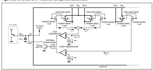
Figure 20. Overcurrent Protection Simplified Schematic
