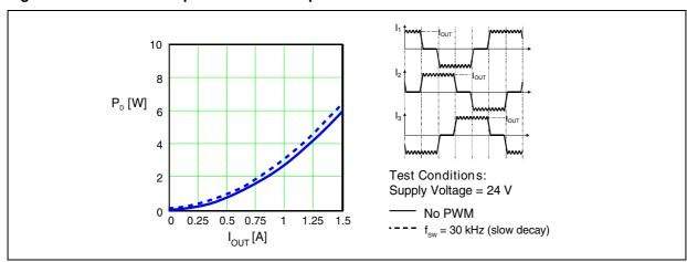
Figure 25. IC Power Dissipation versus Output Power.
