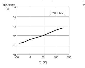
Figure 20. Gate-drive clamp vs. Ti
