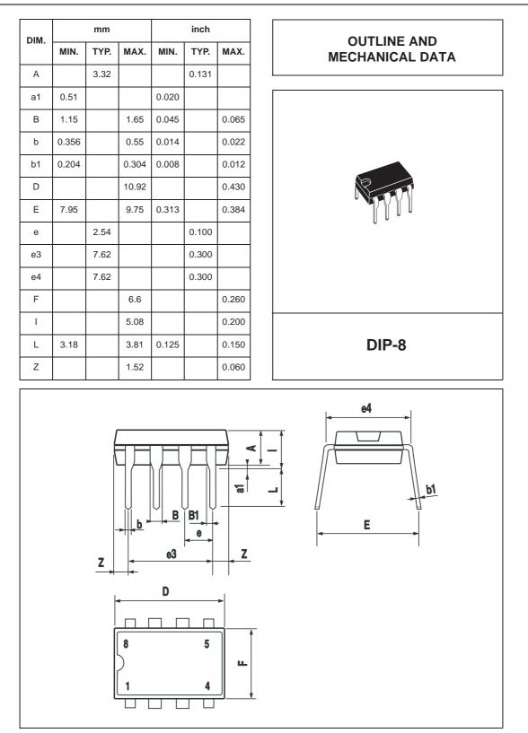
Figure 27. DIP-8 Mechanical Data & Package Dimensions
