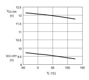
Figure 7. Vcc Zener voltage vs. T<sub>i</sub>
