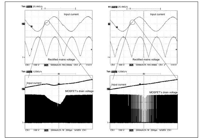
Figure 22. THD optimization: standard TM PFC controller (left side) and L6562 (right side)
