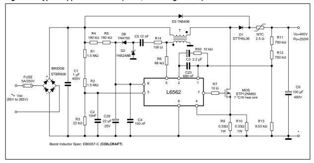
Figure 23. Typical application circuit (250W, Wide-range mains)
