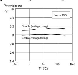
Figure 24. Standby pin dropout vs. Tj
