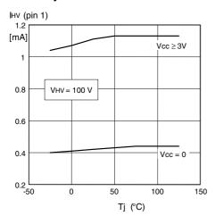
Figure 6. High-voltage generator output (Vcc charge current) vs. Tj
