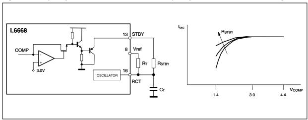
This is done by adding an external resistor R<sub>STBY</sub> between pins RCT (#16) and STBY (#13), which activates the circuit shown in figure 38.
