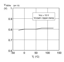
Figure 20. Disable level on current sense vs. Tj
