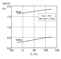
Figure 30. UVLO saturation vs. Tj
