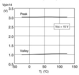
Figure 19. Current sense clamp vs. Tj
