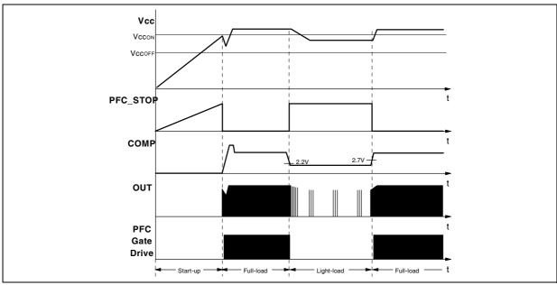
Figure 44. Operation after DIS pin activation: timing diagram
