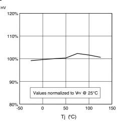
Figure 9. High-voltage generator Vcc restart voltage vs. Tj
