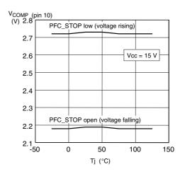
Figure 23. Standby thresholds vs. Tj
