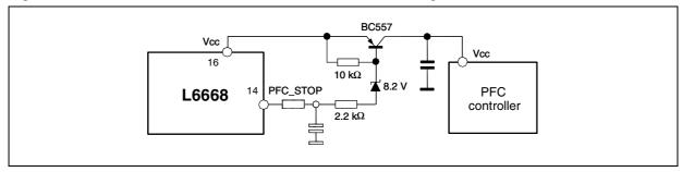
Figure 43. Operation of PFC\_STOP function
