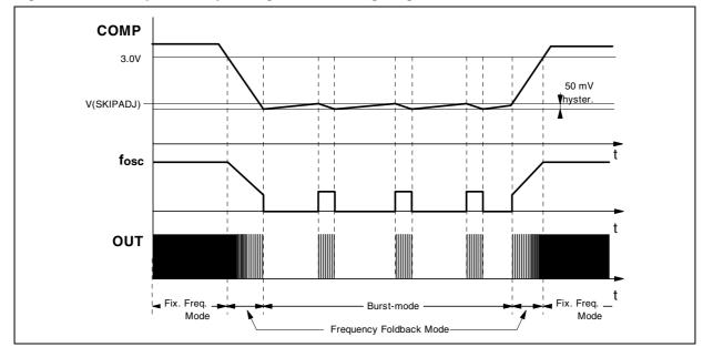
Figure 40. Load-dependent operating modes: timing diagram
