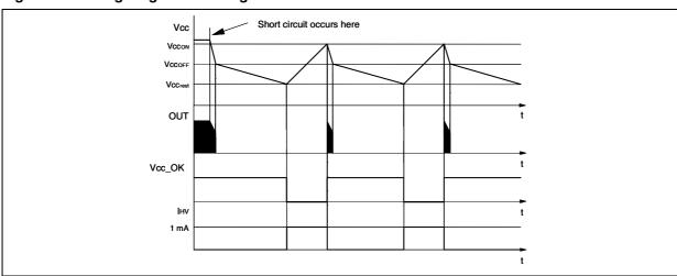
Figure 37. Timing diagram showing short-circuit behavior
