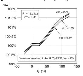
Figure 18. Oscillator ramp vs. Tj
