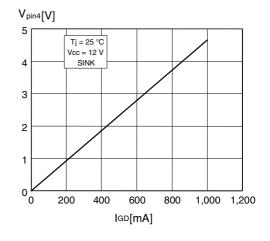
Figure 33. Gate-drive output high saturation
