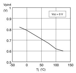
Figure 31. Gate-drive clamp vs. Tj
