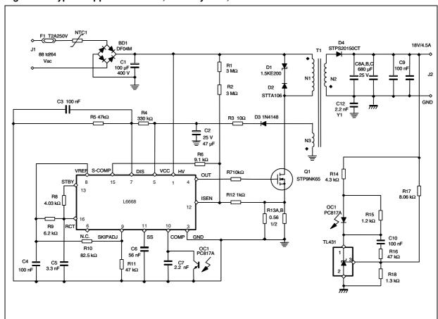
Figure 46. Typical Application: 80W, WRM flyback; Electrical Schematic
