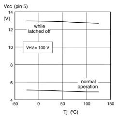
Figure 10. IC consumption vs. Tj
