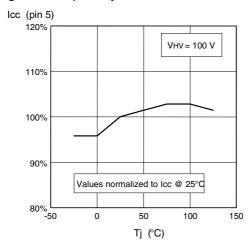
Figure 7. High-voltage pin leakage vs. Tj
