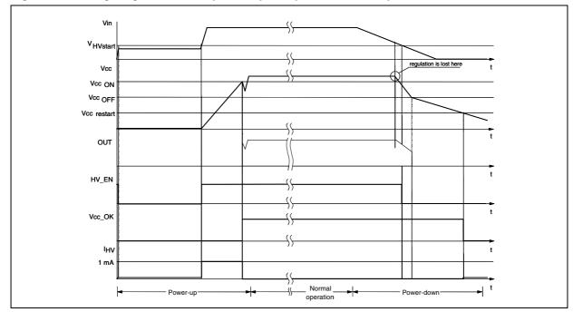
Figure 36. Timing diagram: normal power-up and power-down sequences
