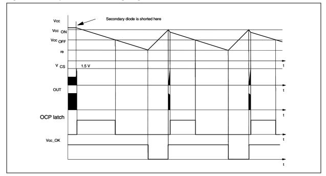
Figure 41. Hiccup-mode OCP: timing diagram
