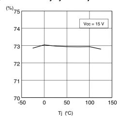
Figure 17. Oscillator frequency vs. Tj
