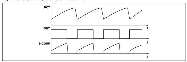
Figure 45. Slope compensation waveforms
