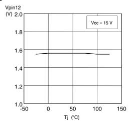
Figure 21. Reference voltage vs. Tj
