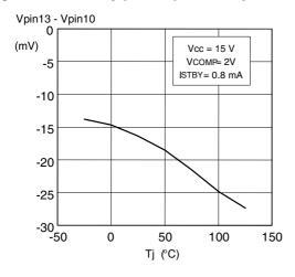
Figure 25. DIS threshold vs. Tj
