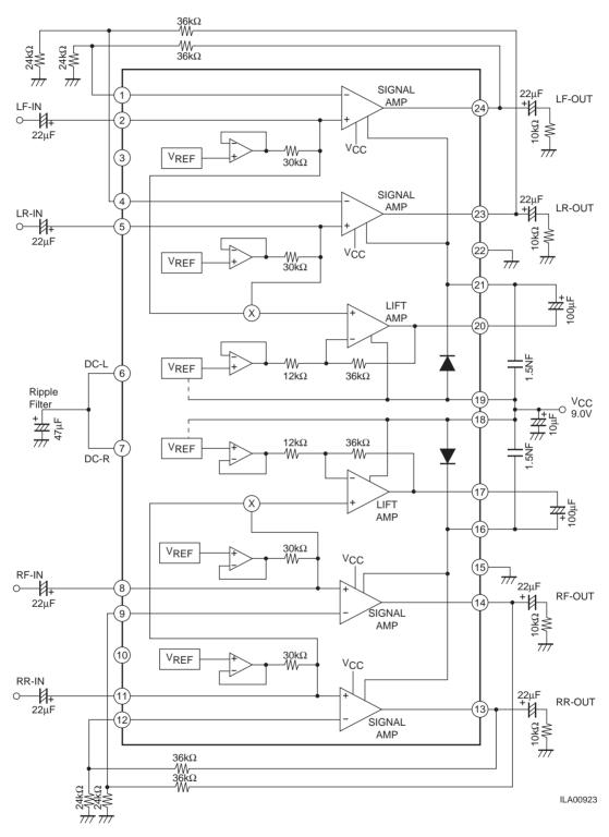
Note: We recommend using resistors with tolerances of 1% or better for the 24 k $\Omega$  and 36 k $\Omega$  feedback resistors.
