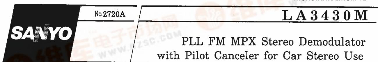
The LA3430M (MFP-16 package version of LA3430) is an MPX IC for FM car stereo use. It contains the VCO non-adjusting function, skip noise eliminating function, and pilot cancel function.
