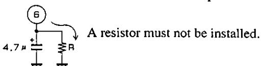
A resistor must not be installed.
