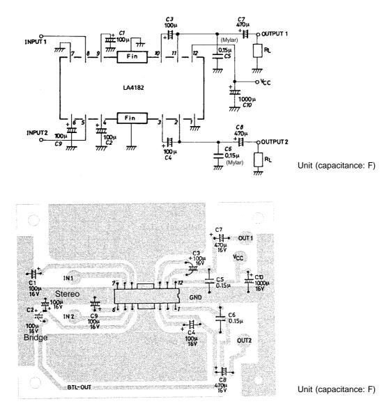
Example of printed pattern (bottom view) for use in stereo, bridge amplifier applications :  $60 \times 80 \text{ mm}^2$
