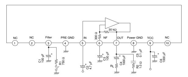
\* For Muting, add a resistor between pin 3 and GND. 750  $\Omega$  for the LA4266/67/68, 200  $\Omega$  for the LA4276/77.
