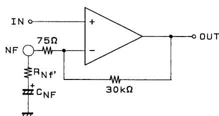
The voltage gain  $VG$  can be lowered by connecting an external resistor in series between the NF pin (pins 8 and 14) and  $C_{NE}$ .
