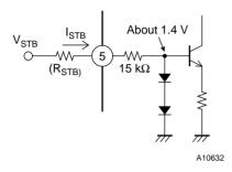
Pin 5 in this IC is the standby pin, and applying a voltage of 2.0 V or higher will activate this function. The pin 5 influx current for an applied voltage of 5 V will be about 240  $\mu A$ .
