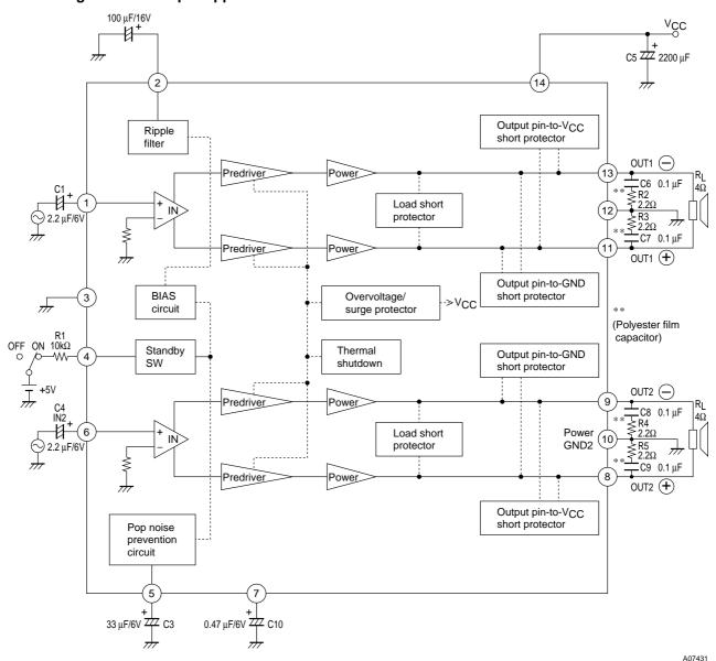
**Block Diagram and Sample Application Circuit**
