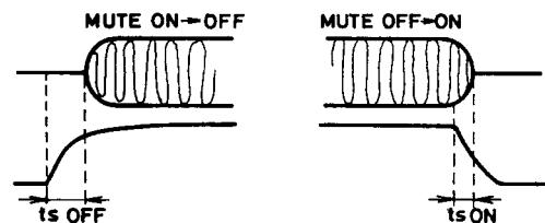
The mute ON/OFF switching waveforms are shown in the figure above. The settling time  $t_s$  is determined by the capacitor  $C_r$  connected to pin 16. The recommended value of  $C_r$  is 1  $\mu\text{F}$ . If the value used is less than 1  $\mu\text{F}$ , pop noise will increase.
