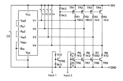
$$\label{eq:VCC} \begin{split} V_{CC} - V_{EE} &= 35 \ V, \ R_X = 8 R, \ C1 \ to \ C4 = 10 \ \mu F, \ C5 = 33 \ \mu F, \ All \ resistors \ must \ be \ rated \ 1 \ W \ or \ higher. \\ TR1 \ to \ TR4; \ 2SA984 \qquad Rank \ E \ or \ F \\ TR5 \ to \ TR9; \ 2SC2274 \qquad Rank \ E \ or \ F \end{split}$$
